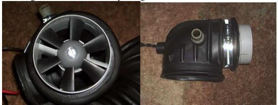
Including with the kit is a wiring kit. As can be seen from the pictures, the fan is operated by a momentary switch mounted to the throttle body.
